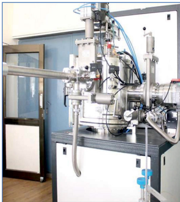
Qubit-Cavity Systems (L) and Double Angle Thermal Evaporation System (R)
