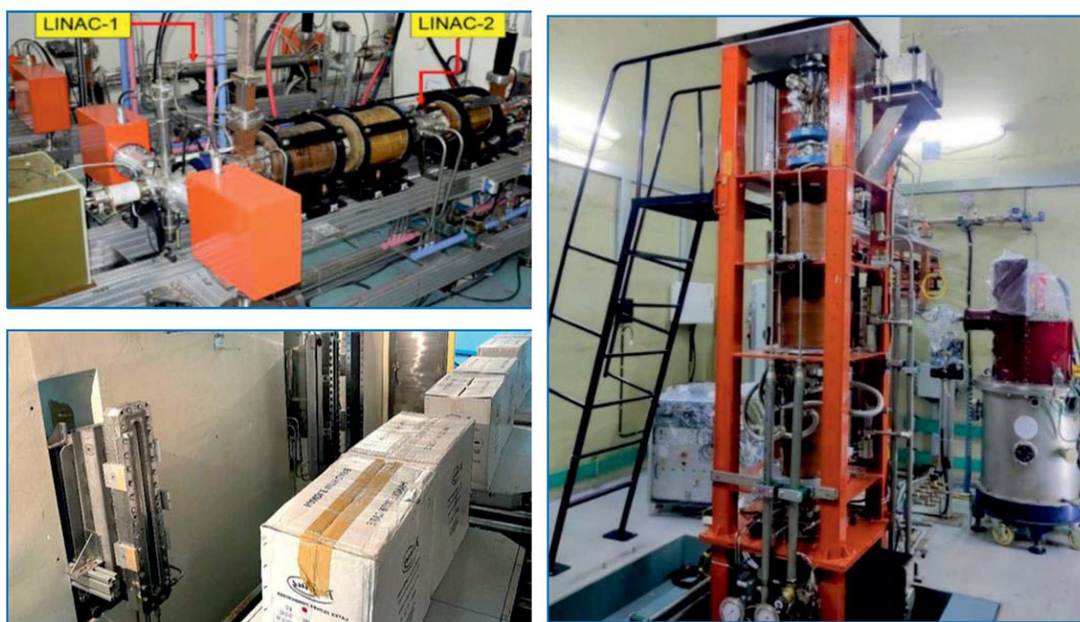
(CCW from Top) 10 MeV LINAC, 6 kW LINAC, KIRTI-1010 (10 MeV, 10 kW) LINAC
